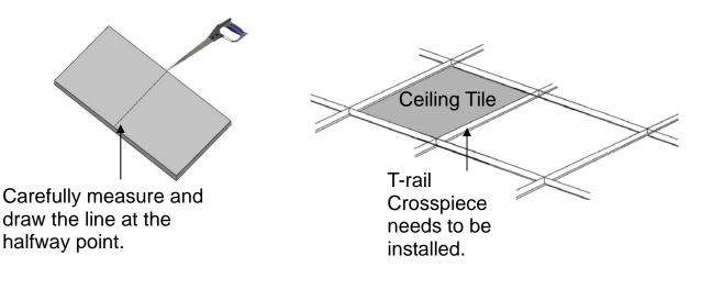
3. Install the T-rail in a rectangular tile – When the ceiling uses rectangular tiles, install the T-rail crosspiece into the ceiling opening up against he cut tile.
