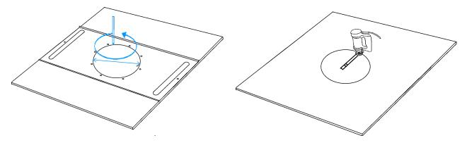
Place the marked tile onto an empty open box or trashcan, to catch any debris. Please make sure to have appropriate clearance for the saw blade and cut the hole with a "plunge' hand or power saw.
